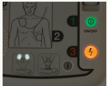
The device will announce whether or not a shock is advised. If shock is advised, there will be a continuous beep and the shock button will flash orange. Press the flashing orange shock button when prompted:
