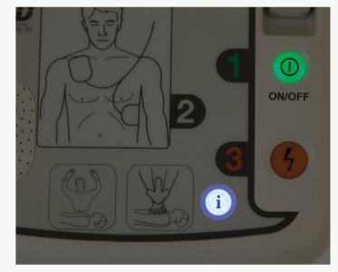
**If no shock is advised,** even if you press the orange shock button, there is no way the device can deliver a shock.
