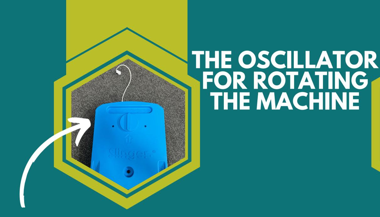
THIS IS THE OSCILLATOR - BASICALLY IT IS WHAT MAKES THE BALL MACHINE ROTATE - PLUG THE WHITE WIRE INTO THE CONTROL PANEL AS PER PREVIOUSE PAGE
